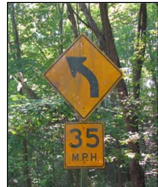
Figure 38. Photo. Low Retroreflectivity sign example.
